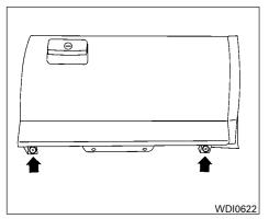
1. Remove the 2 lower glove box screws.
